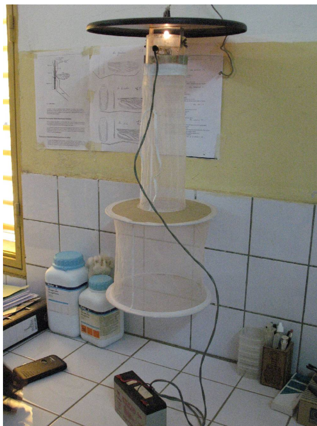
Figure 124: Light trap used for mosquito capture, CRSN Nouna
