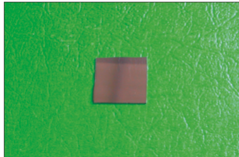
Figure 6.55. Picture of \text{Nd}_{60}\text{Fe}_{30}\text{Al}_{10} film deposited on a Si substrate.
