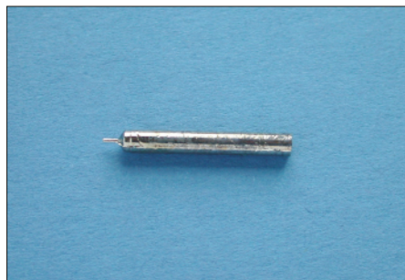
Figure 6.1. Mold cast \text{Nd}_{60}\text{Fe}_{30}\text{Al}_{10} sample cast in a cylindrical mold of 3 mm in diameter and 20 mm long.
