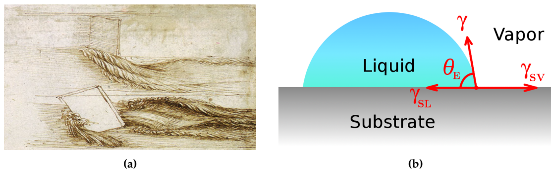
Figure 1.1: (a) Shown is a part from the Codex Leicester by Leonardo da Vinci with a sketch “Studies of water passing obstacles and falling” (ca. 1508). (b) An illustration of the Young equation, connecting interfacial tensions between phases and the contact angle of the droplet, resting at equilibrium on a flat substrate.
