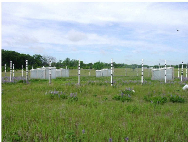
Figure 1 | Photograph showing one of the six FACE rings of the BioCON experiment in secondary successional grassland in Minnesota, USA (Reich et al., 2001a) with four of the 24 portable rain-out shelters temporarily in position above the plots of the precipitation.
