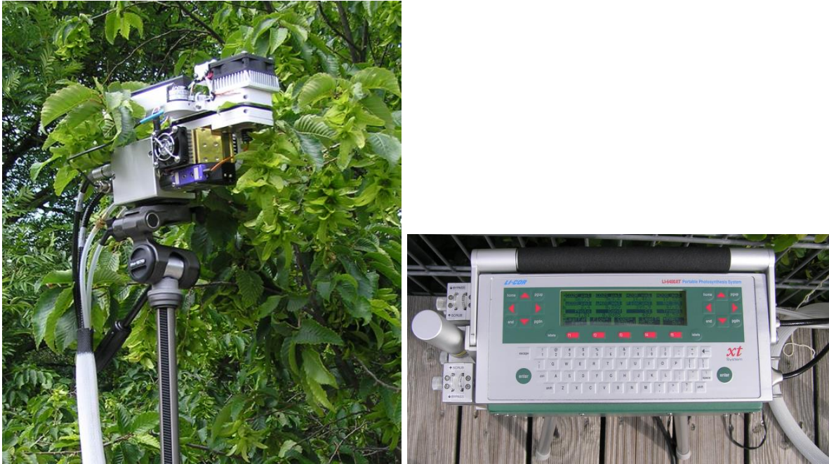
Figure 1.9: The measuring cuvette (left) and the control unit (right) of the Li6400xt. In the cuvette, a leaf of C. betulus is inserted. The IRGAs are located close to the cuvette. Left of the control unit, the gas mixing unit can be seen as well as the humidity adjuster.
