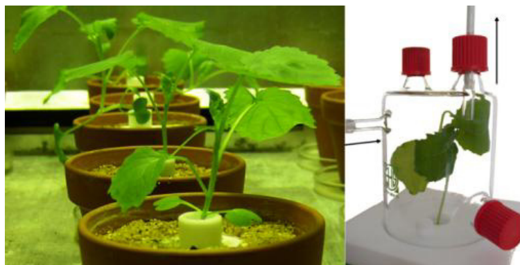
Fig. AI-2: Brassica napus plants grown in a PTFE-collar (left) and inside a glass vessel during sampling (air gets lead into the vessel and sucked through a TDS-Tube (right))
