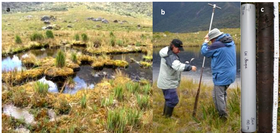
Fig. 2.1 a.b.c. Example of areas where the cores were taken, sediments extraction using Russian corer, sediment stored in 50 cm tube, respectively.
