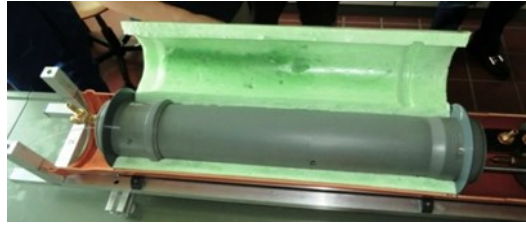
Figure 2.2: Installation of isothermal insulation; In gray is the column chamber surrounded by insulation (green) and coating (orange).
