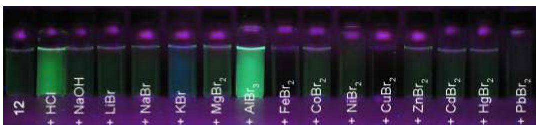
Figure 2-31: Behavior of 12 with respectively 10 eq. of acid, base or metal bromide in MeOH.
