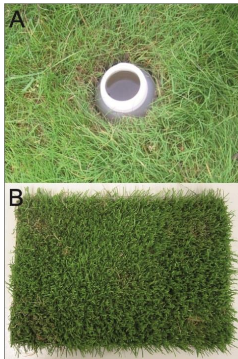
Figure 3-2: Field devices used to sample inundation sediments. (A) One litre LDPE-bottle buried in the marsh soil. (B) Mat of synthetic turf, fixed with steel nails onto the ground.
