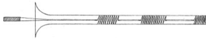
Figure 1.4: Localization of turbulence. At low Re the flow is spatio-temporally intermittent, consisting of an irregular sequence of laminar and turbulent patches in the streamwise direction. Reynolds called the turbulent patches ‘ flashes of turbulence ’, nowadays there commonly referred to as ‘puffs’. The figure is a public domain and taken from Reynolds (1883).
