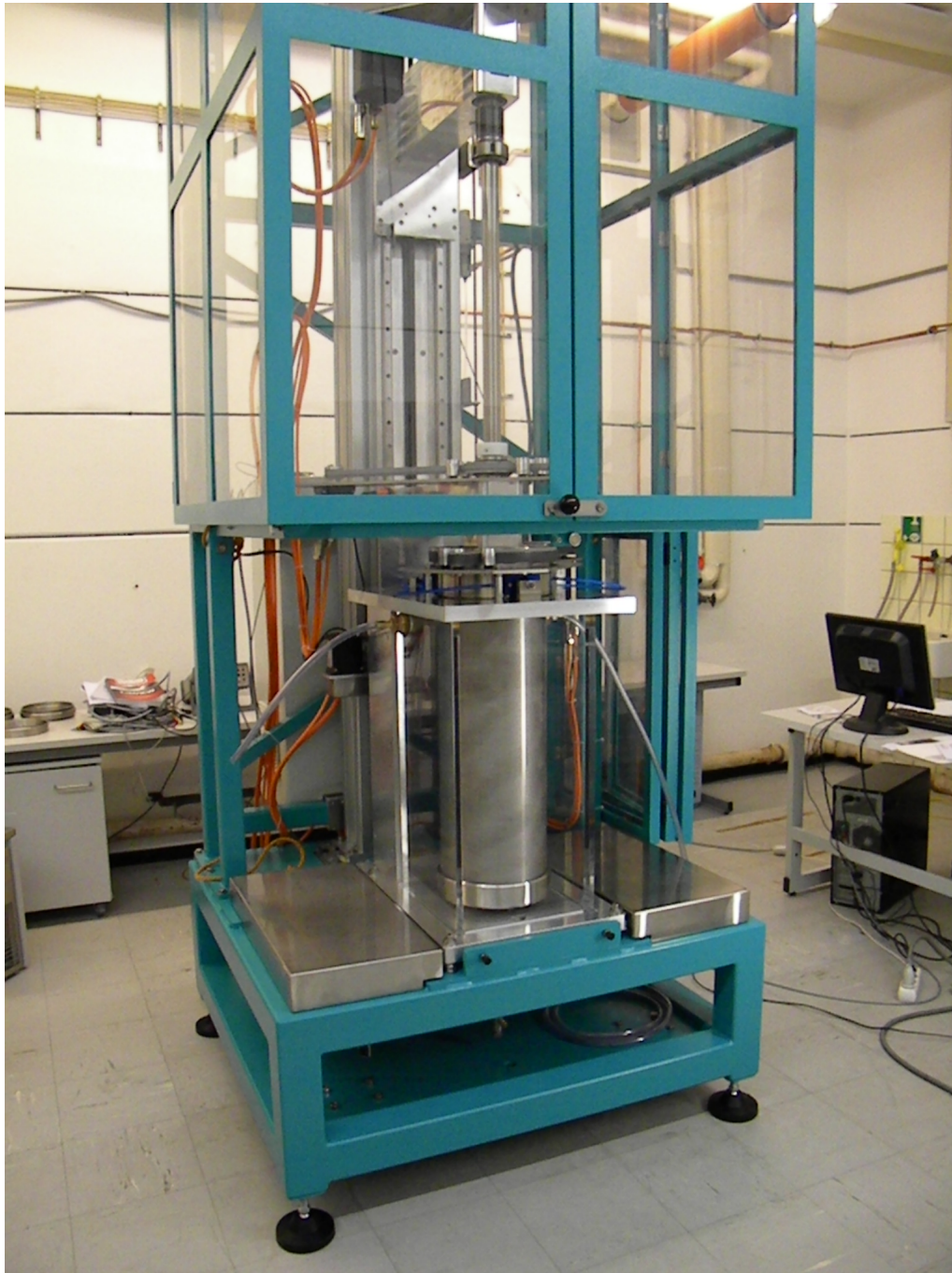
Figure 3.2: The Taylor-Couette device consists of three main assembly groups. The first group consists of the cylinders, the bottom endplate and the acrylic box (see Fig. 3.1). The second group allows an axial movement of the top endplate during measurements over the full length of the cylinders. It consists of a heavy-lift profile along which two massive sledges can be moved, that bear the top endplate and the top of the inner cylinder (see Fig. 3.5). The third assembly group is a stiff frame (here shown in green) on which the first and second assembly groups are mounted and aligned with respect to each other.
