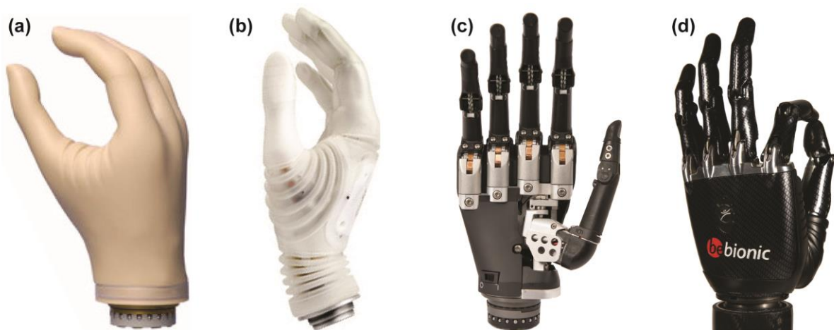
Figure 2: Examples of myoelectric hands commercially available: The Ottobock DMC Plus (a) is a typical prosthetic device with hand open/close and rotation that is widely used in clinical practice. In contrast to this the Ottobock Michaelangelo Hand (b), Touchbionics iLimb (c), and RSL Steeper Bebionic (d) are more advanced prosthetic hands, providing additional functions like the independent control of single fingers. Although the four models shown differ in complexity and components, with some offering different grip patterns (adjustable by external means), all are based on the simple and sequential control scheme, including its limitations for the prosthetic user.
