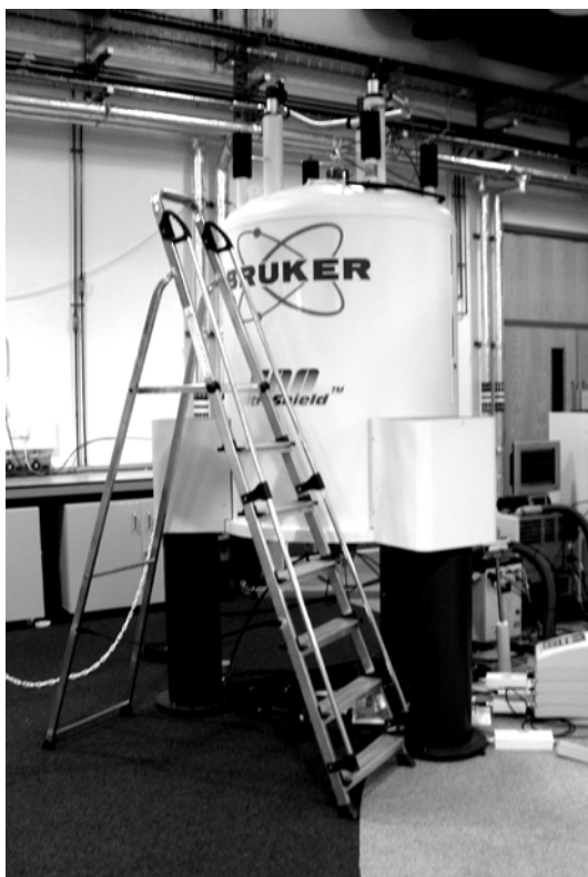
Fig. 8. 500 MHz (11.7 T) spectrometer at University of Warwick.
