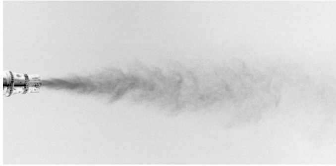
FIGURE 7.3: Inverted greyscale image of the particle jet produced by the airbrush system.
