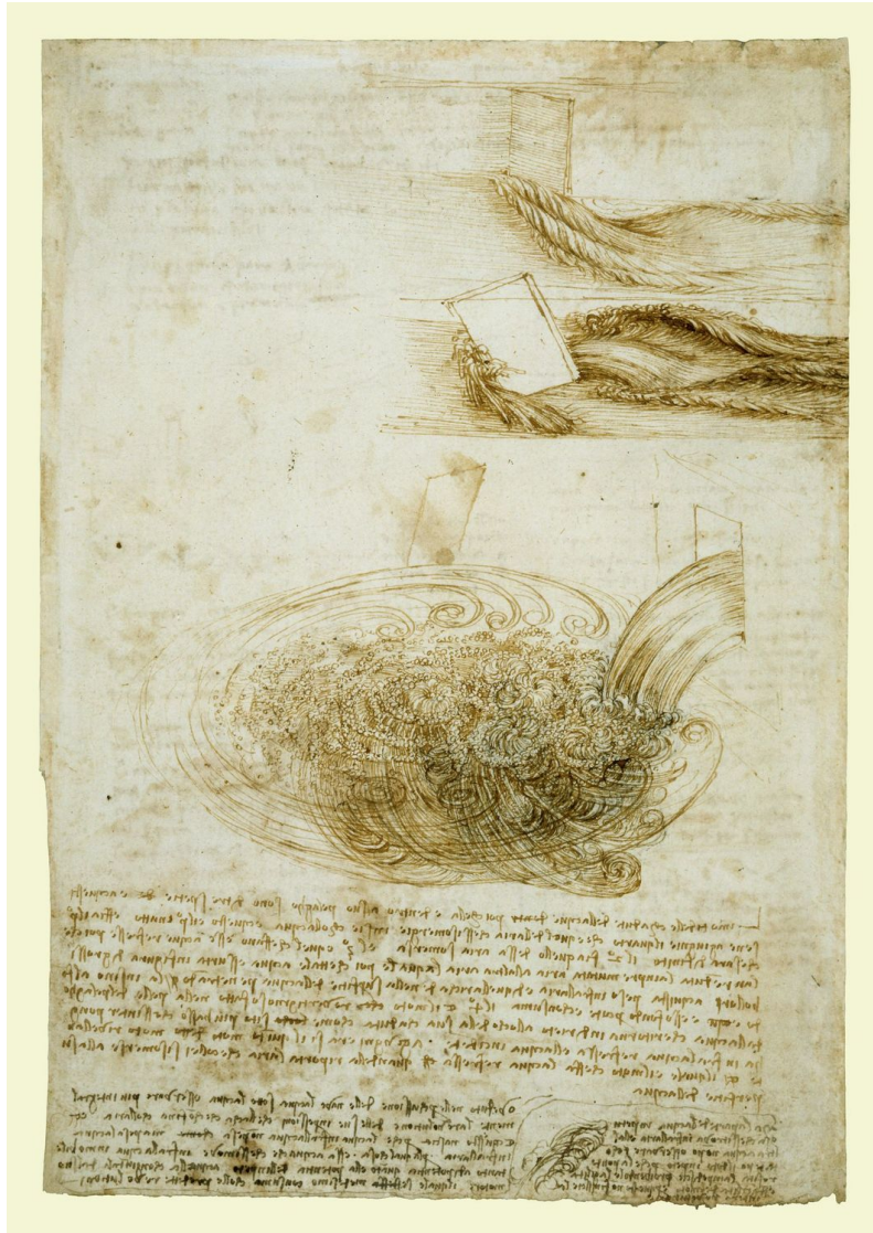
FIGURE 2.7: This most elaborate of Leonardo's sheets of water studies investigates two basic themes. The first, in the upper two drawings, is the flow of water past a planar obstruction. Below, Leonardo shows the fall of a stream of water from a sluice into a pool, a lucid and highly sophisticated study in which the multiple layered vortices are seen extending far below the surface, each welling current giving rise to concentric circles of bubbles that expand across each other without interference. Leonardo da Vinci (approx. 1510) (source: Caption and image taken from Royal Collection Trust / ©Her Majesty Queen Elizabeth II 2014 [135]).
