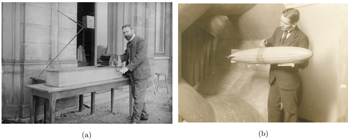
FIGURE 2.8: (a) Prandtl in front of the water channel in Hanover (1904); (b) a model of the Zeppelin Airship LZ120 'Bodensee' in the wind tunnel II in Göttingen (1920) (source: [36] 10 ).
