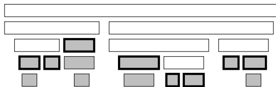
(a) For the first machine, a class \mathcal{C}^1 (grey) of the interval partitioning is chosen uniformly at random. The intervals in I^1(\mathcal{C}^1) are highlighted with a black frame.
