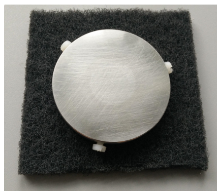
Figure 3.20: Stainless steel bottom plate of rheometer.
