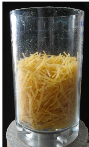
Figure 5.4: Experimental setup: Packing of spaghetti (rods) in a cylinder.
