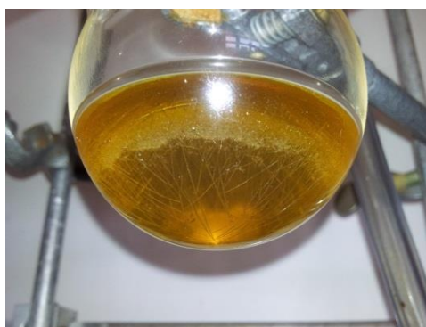
Figure 2-17: Needles of CpCs which were crystallized at ambient temperature in THF solution.
