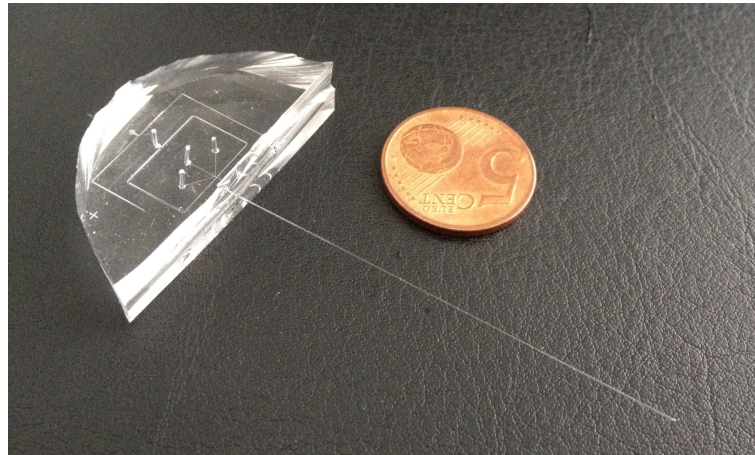
Figure 3.4.: Photograph of the assembled droplet device. The composite PDMS-Quartz device is placed with a 5-cent coin to highlight its size and portability.
