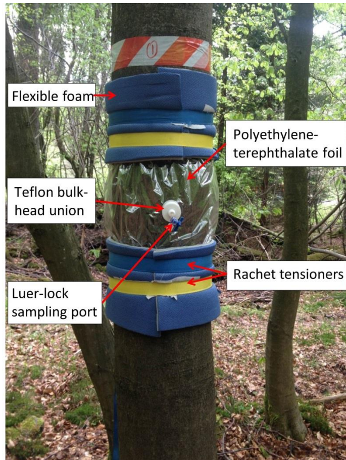
Figure 1. Oven bag chamber method, used to measure in situ stem N 2 O fluxes.
