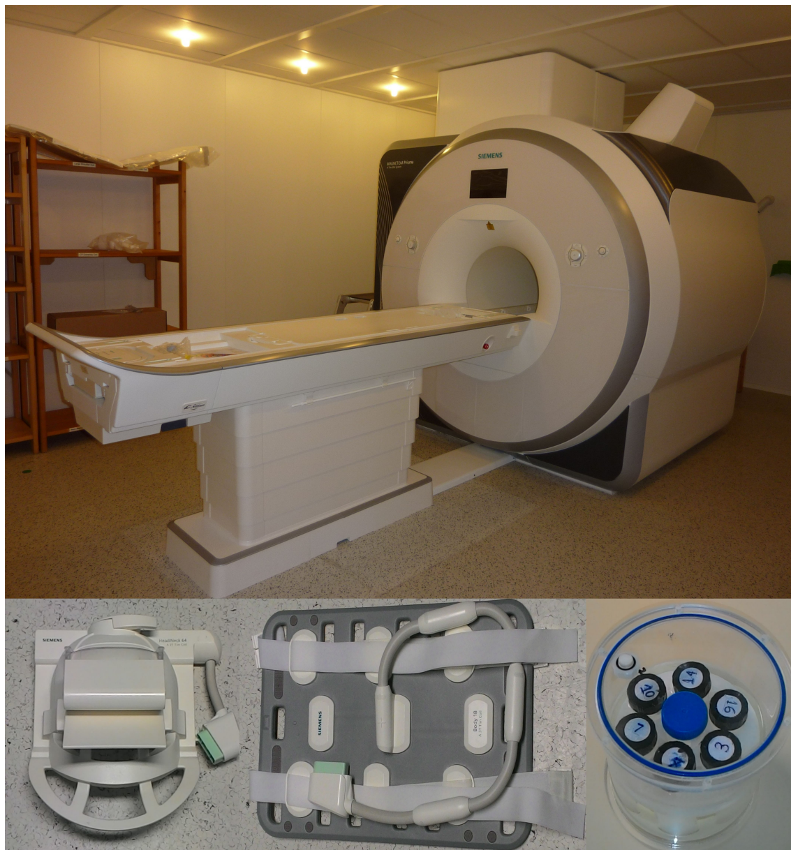
Figure 2.12: (Top) MRI system, (bottom left) 64-channel head coil, (bottom middle) 18-element thorax coil and (bottom right) a commercial T_1 phantom used in this thesis.
