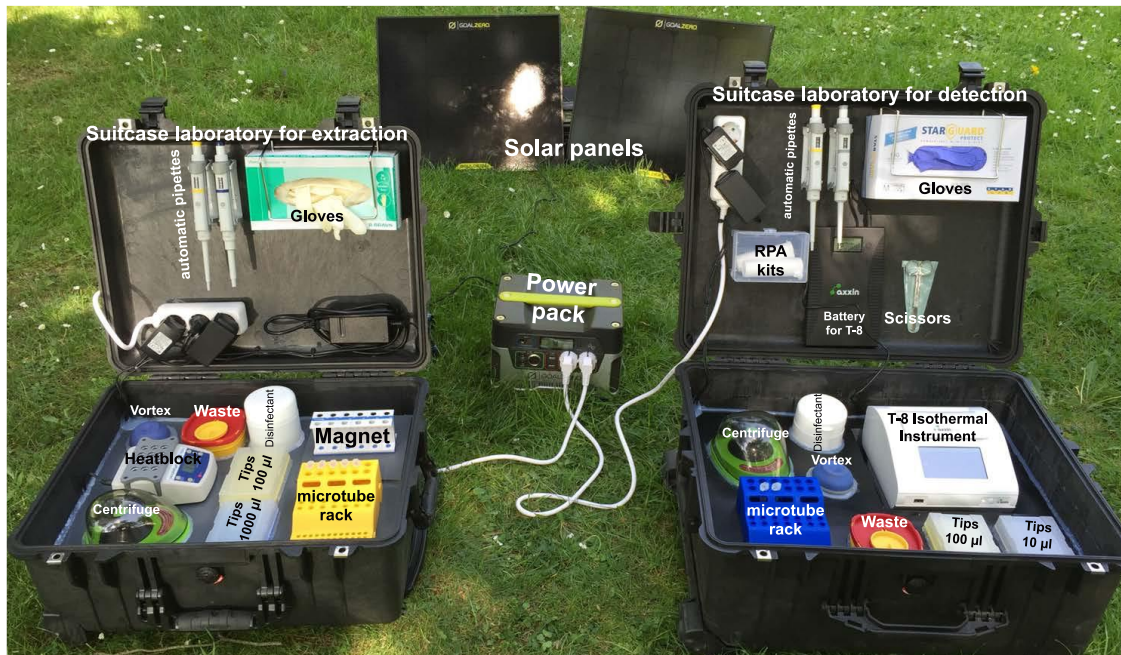
Figure 12: The mobile suitcase laboratory. The mobile setup consists of two suitcases, one for nucleic acid extraction (left suitcase) and another for detection (right suitcase), which contains all reagents and equipment for the detection of the nucleic acids of infectious agents using RPA technology. All reagents used in the mobile laboratory are cold-chain independent and powered by solar battery, making it ideal for low-resource settings (Division of Microbiology and Animal Hygiene, Georg-August-University Göttingen)
