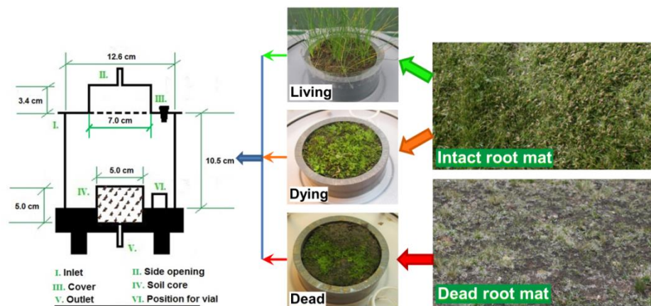
Figure SV-1: Longitudinal section of chamber (left) and origin of three Kobresia root mat types (right). “Living” = living root mat; “Dying” = dying root mat; “Dead” = dead root mat.
