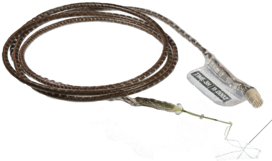
Figure 2.2: Overview of complete TIME array - The TIME array is connected to 50cm of spiralled wire, coated in silicon and ends in a 16-pin Omnetics connector. A thin needle, which is used to pierce the nerve and thread the array through, is attached to the end of the TIME array with a suture wire.
