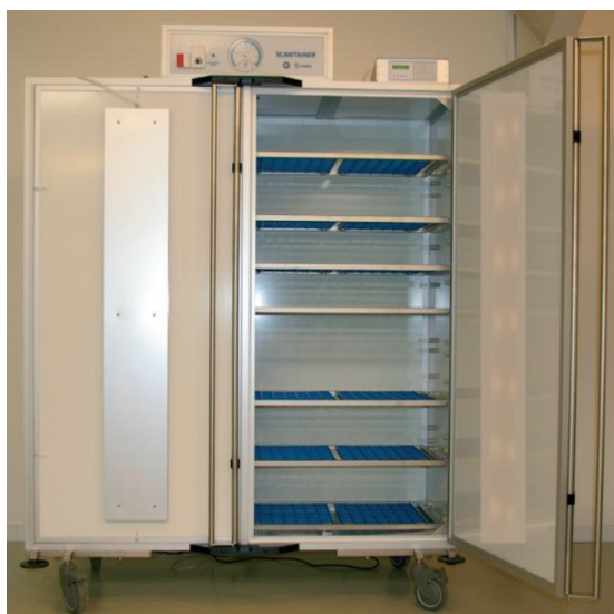
Figure 4: Dark exposure in a Scantainer (Scanbur Technology, Denmark) with light adjustment kit. The animals were raised in the Scantainer from birth in complete darkness. The lights in the animal room and in the Scantainer were always turned off. (Figure modified from www.scanburtechnology.com/fileadmin/SCBTechnology/Brochure/Scantainer_light_adjustment_kit_03.2011.pdf ).
