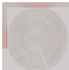
Fig. 5. Application of the circular Sobel operator to the tree disc of Fig. 2. Problematic edges caused by cracks and branches as well as noise are removed.
