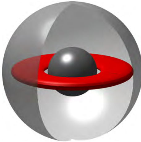
Figure 3.7: The radial jet that emergence due to rotation of the inner sphere when the outer boundary rotates very slow or is stationary. Shown here are isosurfaces of radial velocity, u_r , for \Delta\Omega = 1000 and E = \infty .
