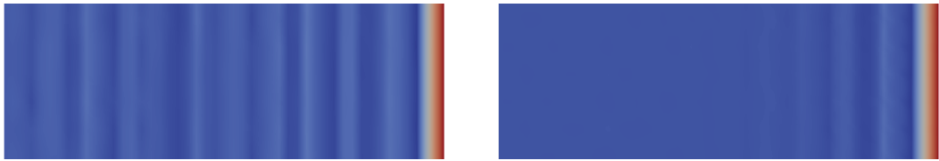
Figure 5.8.: Temperature segment x \in [0, 1] , y \in [0.35, 0.65] at t = 0.005 in case of \mathbb{Q}_2/\mathbb{Q}_1 elements (left) and \mathbb{Q}_2^+/\mathbb{Q}_1 elements (right) for \tau_L^\theta = \|\mathbf{u}_h\|_{\infty,L}^{-2} , (\nu, \alpha, \beta) = (1, 10^{-3}, 1)
