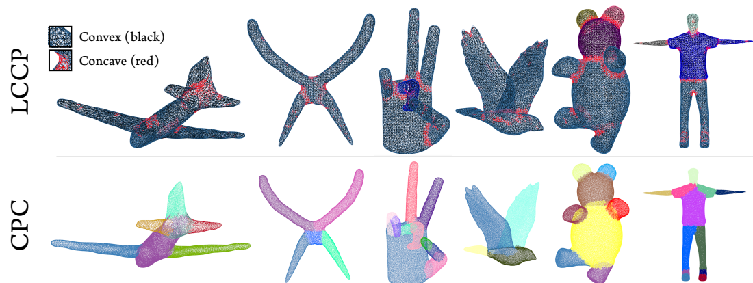
Figure 6.1: LCCP for part-segmentation showing the segmentation and the adjacency graph (top). Problem: Parts of objects are often not completely separated by concavities, which makes LCCP fail. Nevertheless some concavities do exist and hint at part-to-part boundaries. This evidence is used to induce cuts by ways of the CPC algorithm (bottom).
