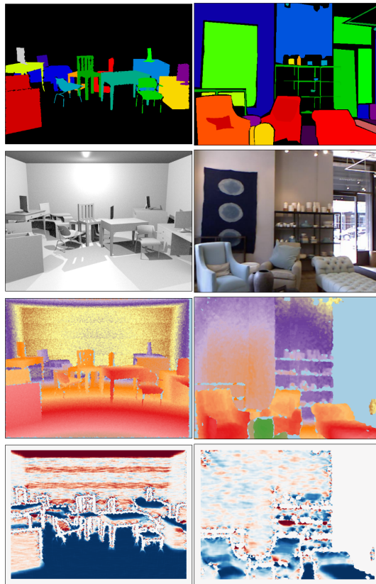
Figure 3. Example of a randomly generated synthetic scene using our rendering pipeline (left) and a scene from the NYUv2 dataset. The rows show A. Ground truth labels, B. RGB Channel, C. Depth Channel, D. Normals calculated using [7]. The left column shows our synthetic data, and the right an image from NYUv2 [12].
