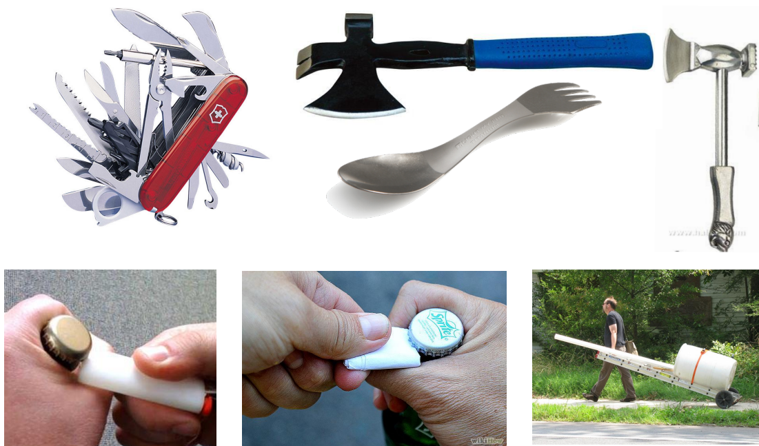
Figure 3.2: Tools which possess multiple functionalities . Top row: Tools specifically designed to be used in multiple applications ( i.e. , multi-tools). Bottom row: Makeshift-replacements with objects being used in a different way from what was intended by the designer.
