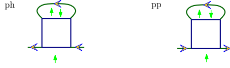
Figure 4.8: Spin configurations in first order for the particle-hole (ph) and particle-particle (pp) channel.
