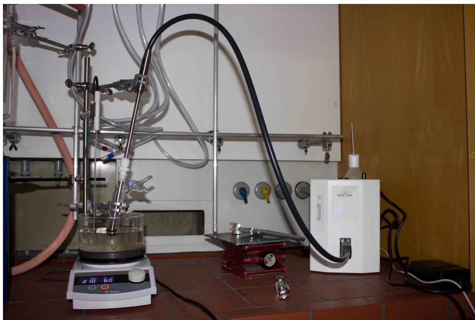
Figure 3.6: Reaction setup using in situ IR Technology.
