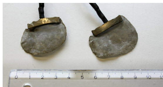
FIGURE 6.7: Mesh electrodes used in the open chest experiments. The shape was individually adapted by cutting the mesh with normal scissors.
