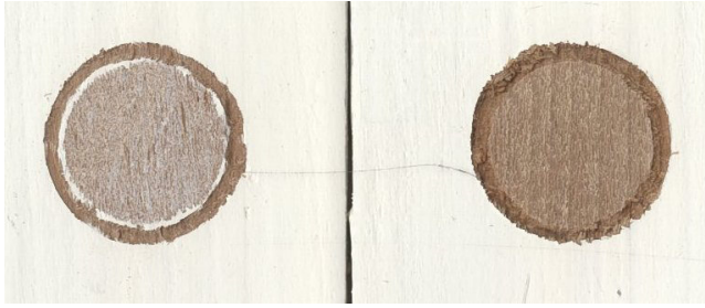
Figure 4: Comparison between untreated control (right) and treated sample after pull-off test.
