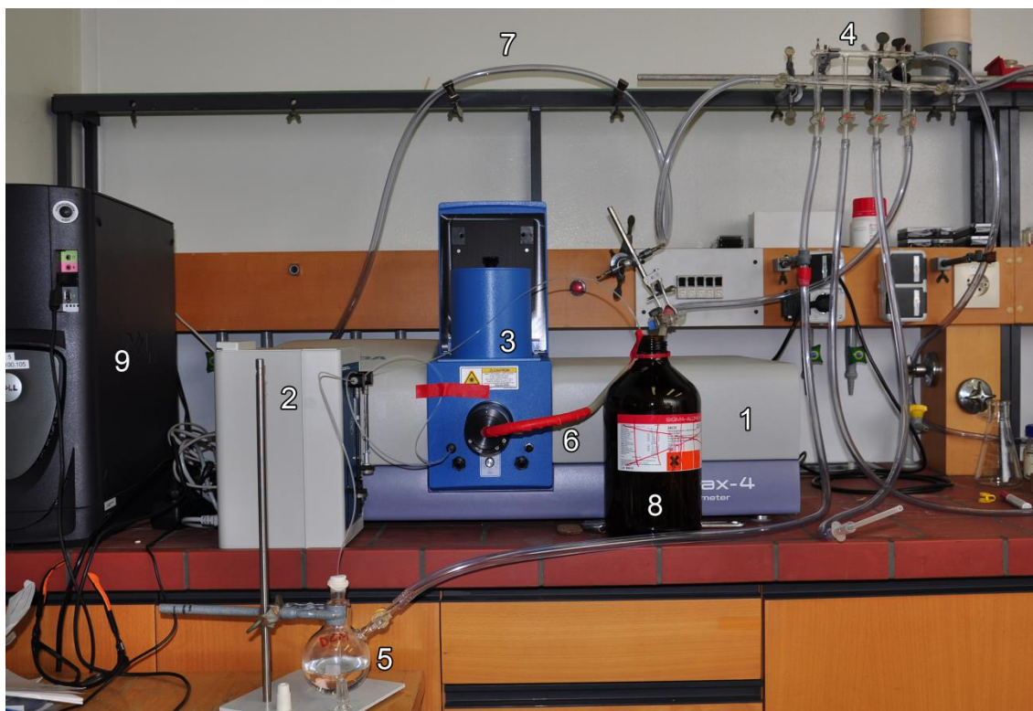
Figure 2-4: Experimental setup. 1: fluorescence spectrometer, 2: titration injector, 3: experimental chamber (with top piece) 4: Schlenk -line, 5: Schlenk -flask containing solvent or analyte solution, 6: light shielded silicone tubing, 7: argon supply, 8: solvent disposal, 9: computer for data collection.
