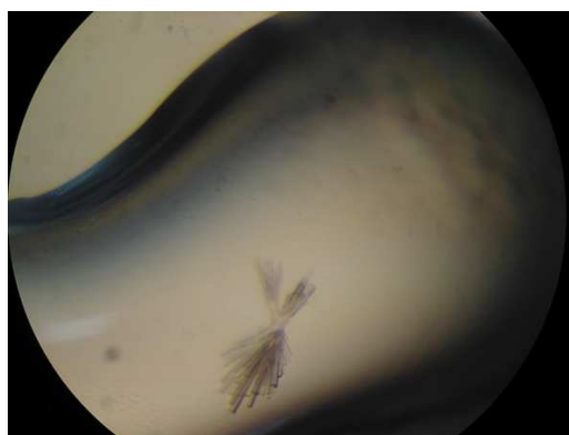
Figure 5.2: Full length PaAtg18 crystal diffracting to 7.7 Å . Crystal was grown in a hanging drop in a 24-wells plate format. The crystallization condition is summarized in Table 5.1.
