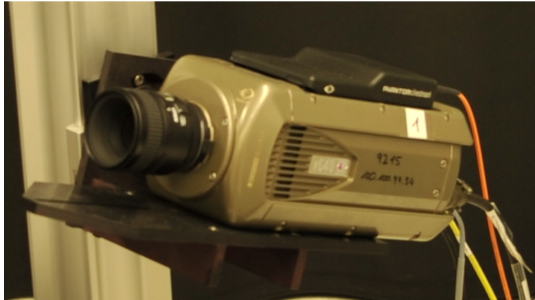
Figure 3.11: Vision Research’s Phantom V640 with CineStream module. The CineStream module provides a fiber output to stream high-speed videos continuously at a data rate of about 1\text{ GB/s} .
