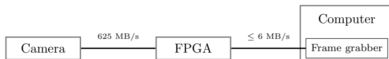
Figure 3.10: Chan et al. (2007) developed an FPGA circuit that receives the camera output, compares every pixel to a threshold and only sends those pixels brighter than the threshold to a frame grabber card. The data rate is reduced by a factor of 100-1000 and therefore the compressed image data can be streamed to the HDD of the computer in real-time.
