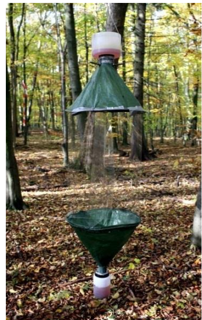
Figure 1 Flight interception trap used to sample beetles along transects extending from forest edges to the interior, across two vertical strata.
