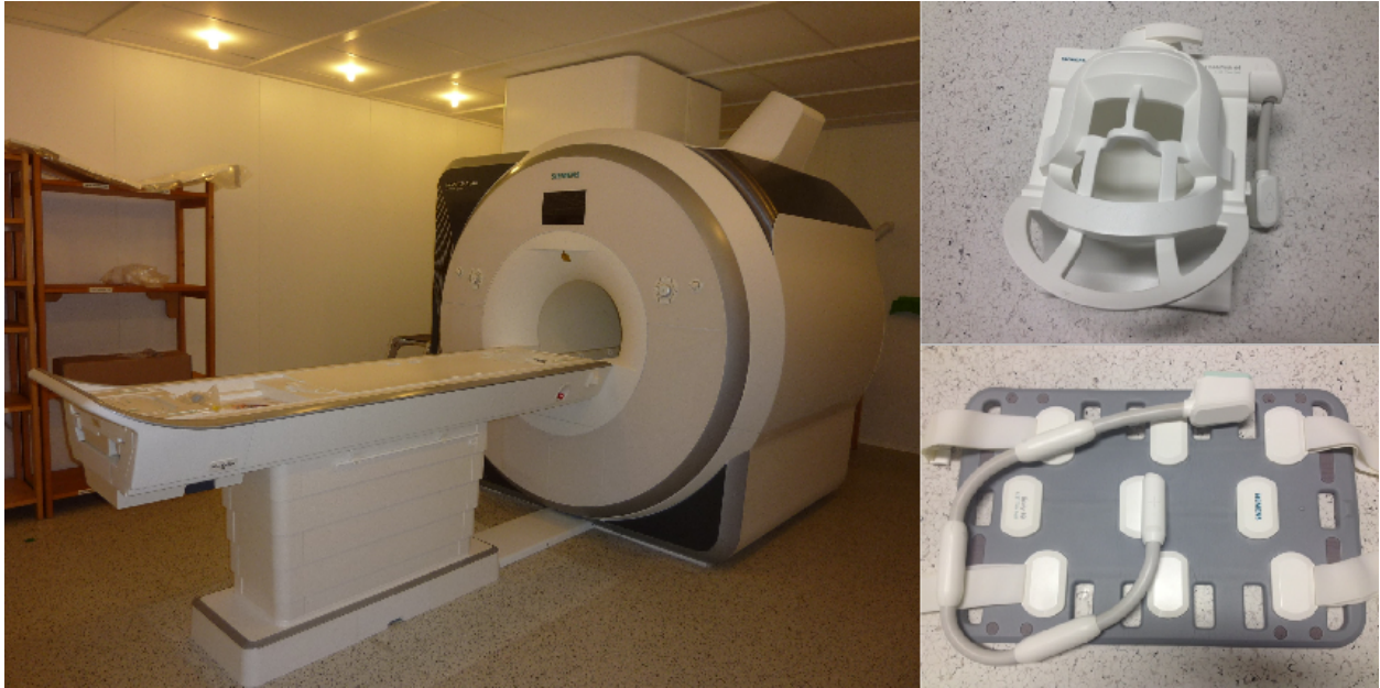
Figure 2.9 (Left) MRI system and (right) receiver coils. (Top right) 64-channel head coil and (bottom right) 18-element thorax coil.
