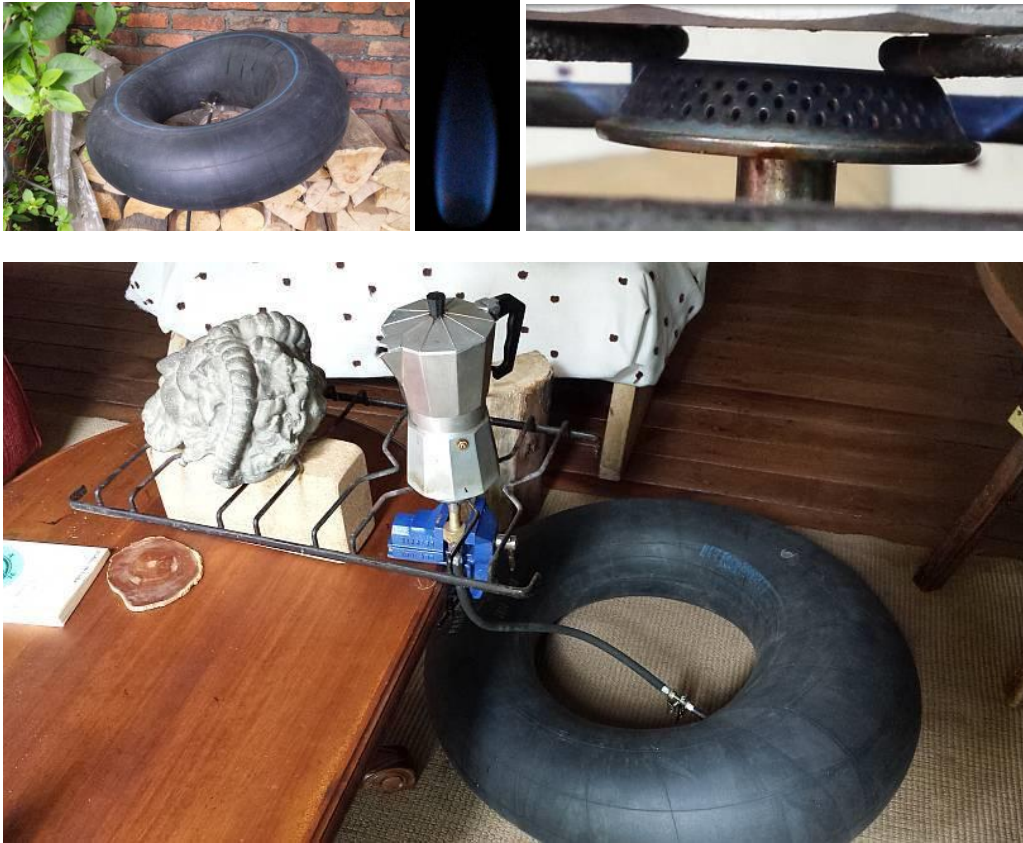
Figure A16: Pictures of an experimental biodigester designed from recycled components and built as experiential work with biogas. a) Steps of building and setting, b) steps of storing and using the biogas.
