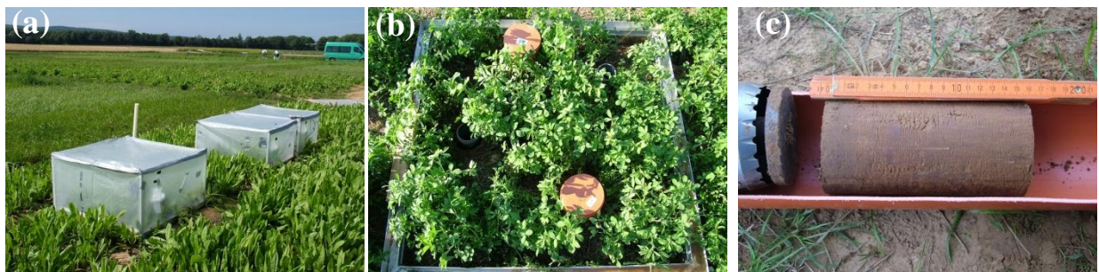
Figure 1.3-2: Chambers that were used for simultaneous in situ ^{13}\text{CO}_2 pulse labeling of three replicate 1 m 2 plots of chicory (a). Alfalfa plot after the pulse labeling with two closed chambers for determining total soil respiration and the contribution of recently assimilated C (b). 15 cm soil cores taken subsequently from the soil surface down to 105 cm depth (c).
