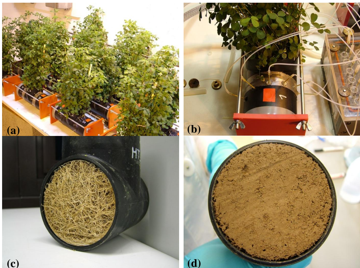
Figure 1.3-4: Alfalfa plants growing in the three-compartment pots used as experimental design in study 2 (a). After the 14 CO 2 pulse labeling of alfalfa soil solution was sampled using micro suction cups (PI Ceramic, Lederhose, Germany) (Göttlein et al. 1996) (b). Alfalfa roots that covered the nylon gauze (c) and the surface of the associated rhizosphere compartment (d).
