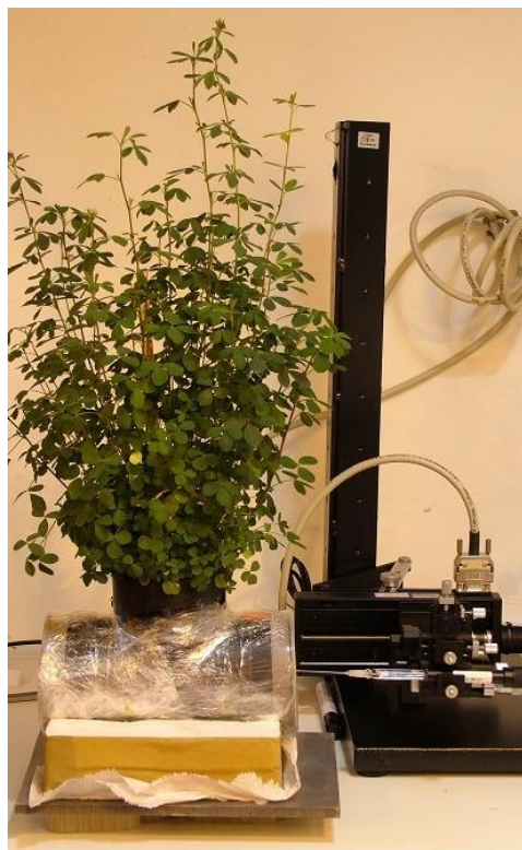
Figure 1.3-5: Realization of the oxygen and redoxpotential measurement in the rhizosphere of alfalfa.
