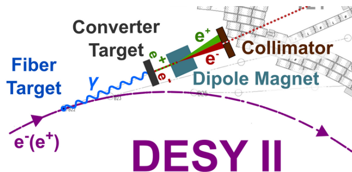
Figure 5.5: Schematic layout of the beam production for test beam measurements.
