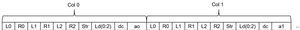
Figure 6.6: Schematic drawing of the sequence of the pixel shift register for two unit cell columns.
