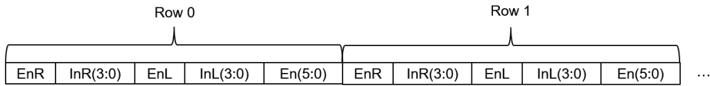
Figure 6.5: Schematic drawing of the sequence of the pixel shift register for two unit cell rows.
