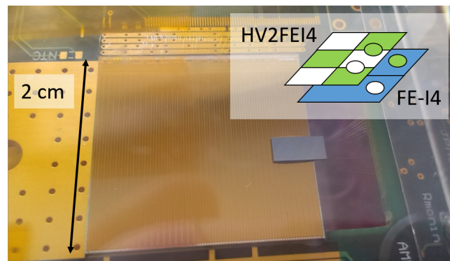
Figure 4.16: Picture of HV2FEI4v2 sensor glued to an FE-I4 readout chip. The inset shows schematic drawing of the subpixel mapping for one unit cell.
