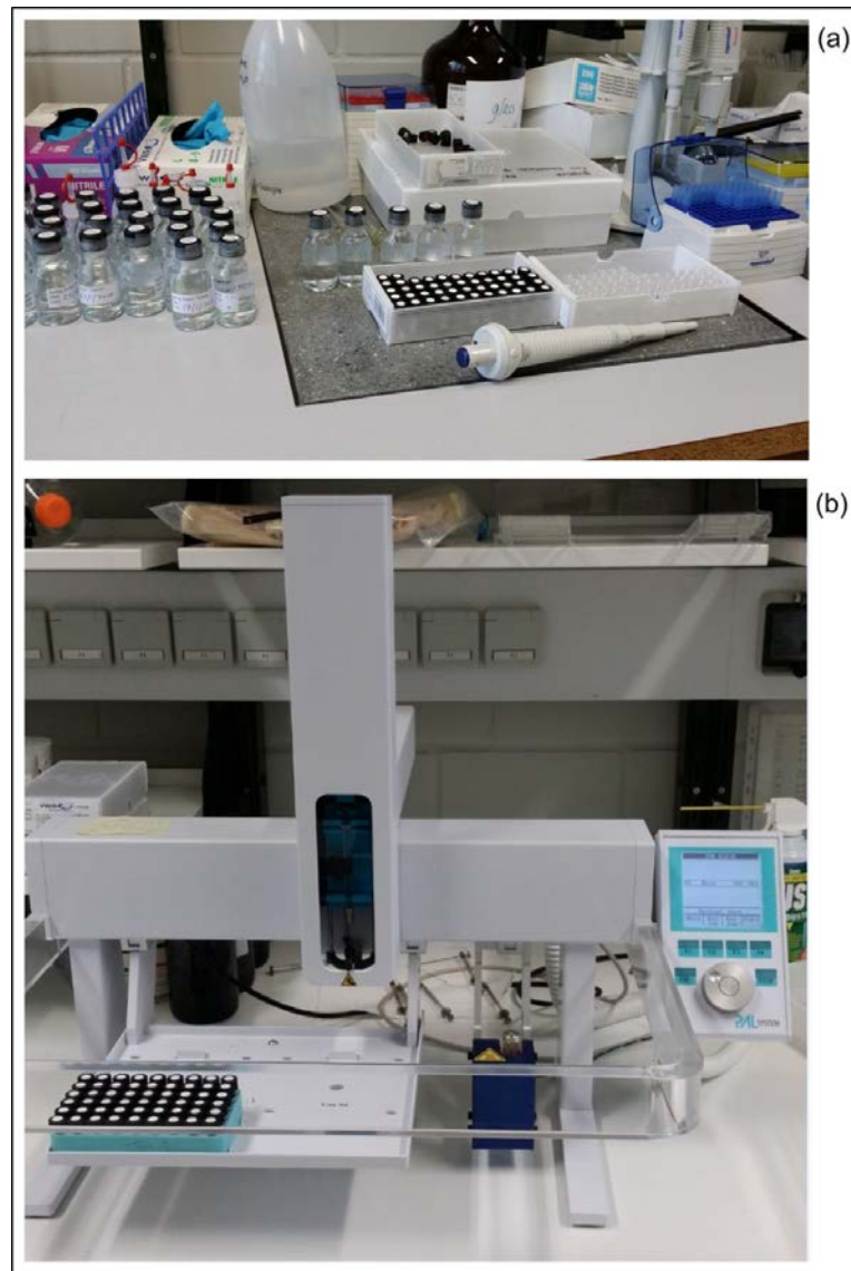
Figure 4-2: Shows (a) samples preparation for analysis, and (b) Liquid Water Isotope Analyzer (LGR, IWA-35-EP) for analyzing \delta^{18}\text{O} and \delta^2\text{H} (photo source: Ibraheem Hamdan).
