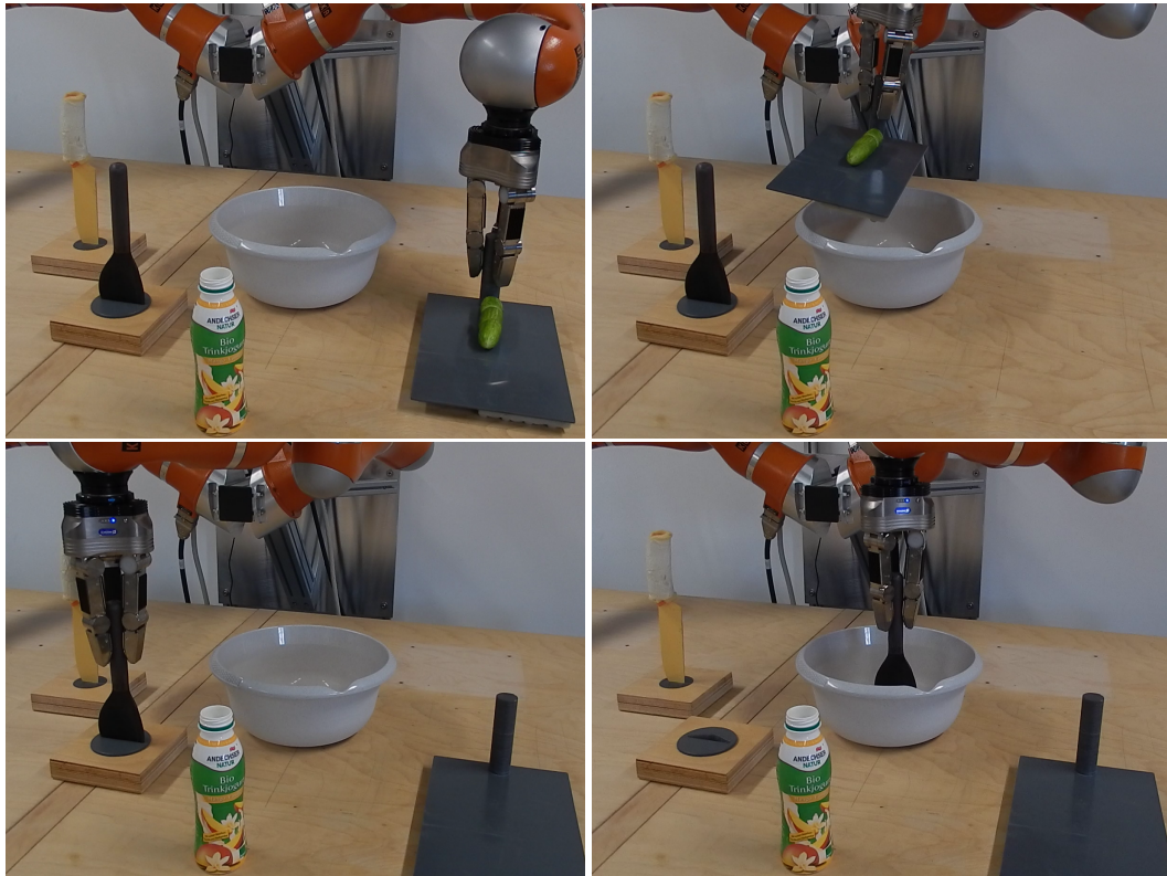
FIGURE 4.10: The execution of chained actions: Unload and Stir by using the spoon.
