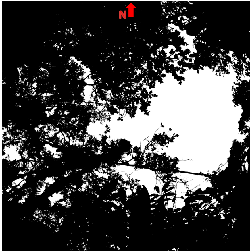
Figure 2.5 Output image produced by Gap Light Analyzer software. The program transformed hemispherical photos to binary images, where pixels in black represent vegetation cover and pixel in white represent the open sky.
