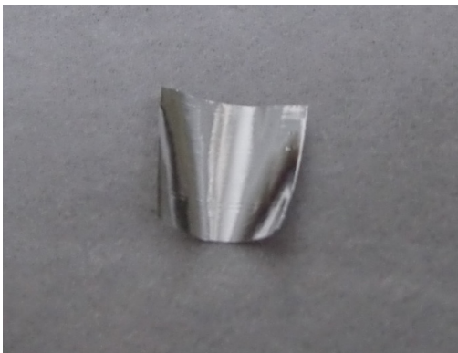
Fig. 5.31 Bulged Pd/Mg/Pd-substrate sample after electrochemical hydrogen loading. (A picture from the Pd-substrate side). The shape of the film remained stable.
