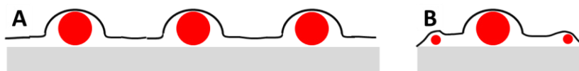
Figure 4.18 Schematical illustration of the polymer shell morphology in self-assembled layers of simple core–shell particles (A) and in planet–satellite nanostructures (B).
