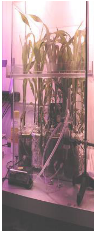
Figure I.2/4 ^{14}\text{CO}_2 pulse labelling of maize with belowground soil microcosms
