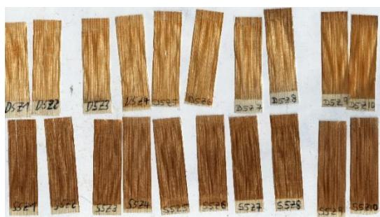
**Fig. 3:** Micro-veneers after 96 h of artificial weathering with demineralized water spray (above) and with seawater spray (below)
