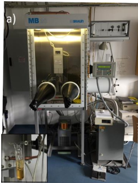
Figure 3.5 (a) Picture of the DMA and glovebox set up in the Mechanical Analysis Laboratory of the 1 st Institute of Physics in Göttingen. (b) Sketch of the different components of the glovebox-DMA set-up.
