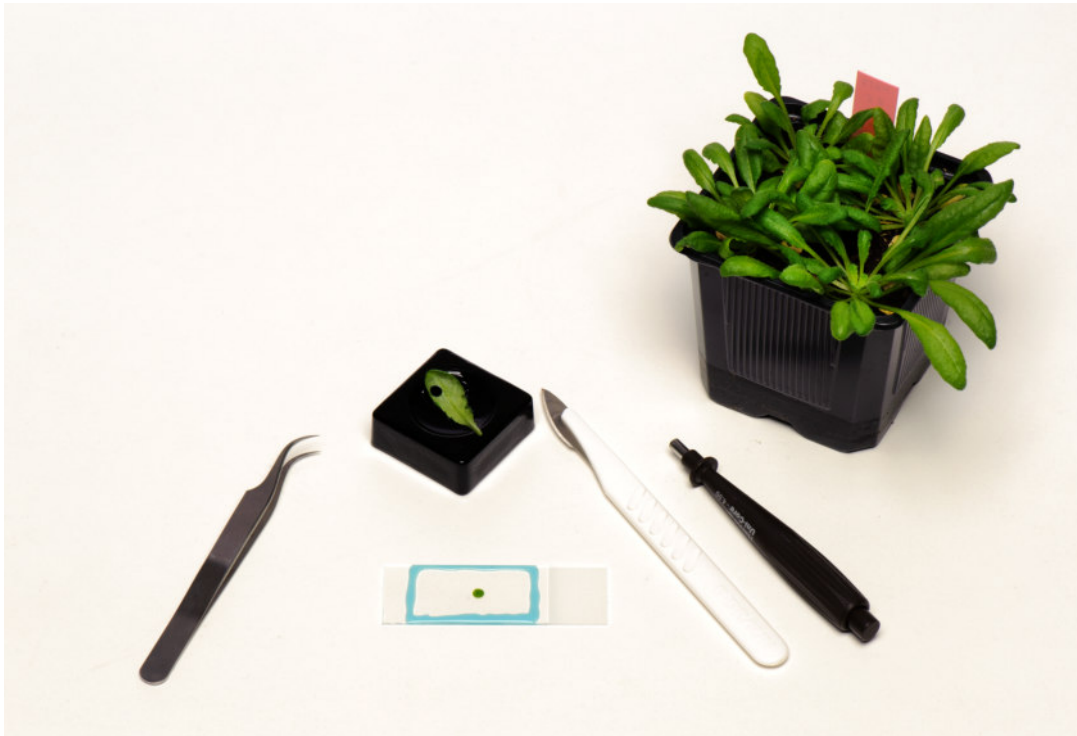
Figure 5.3: Illustration of sample preparation of MAP4-rsEGFP2 expressing Arabidopsis thaliana for imaging of leaf epidermis cells. From green leaves, small pieces of 4 x 4 mm size, were cut out and placed in a drop of PBS, covered with a coverslip and sealed using non-toxic duplicating silicone.
